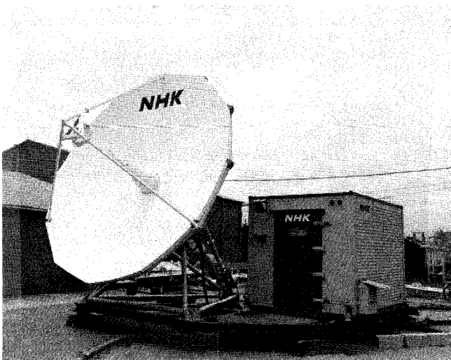
Figure 1 Transportable Transmit and Receive Station of A-Type (TTRS A-Type)
